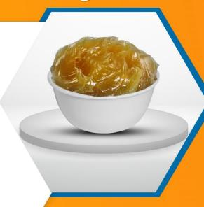
These are molten salts used for Marquenching, Austempering, Hardening, etc. The salt can be selected depending on the operating temperature range required.
